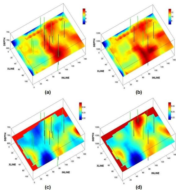
Figure 4: Extensional stress maps at (a) 750 m and (b) 1250 m as well as tangential weakness maps at (c) 750m and (d) 1250m with well track inserts (green - injection &amp; black - production) for reference
