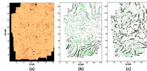
Figure 5: (a) Sample depth slice map of fracture zone indicator (FZI) using seismic and microseismic derived properties (ANN framework), (b) integrated display showing threshold limited FZI with discontinuity at 1000 m and (c) at 1500 m
