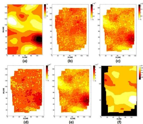
Figure 3: (a)  $V_p/V_s$ , (b)  $\mu$ , (c)  $\lambda$ , (d)  $K$ , (e)  $E$  & (f)  $\sigma$  at 1000m
