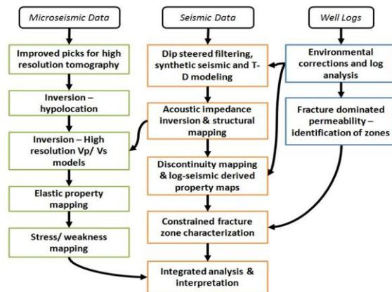
Figure 1: Integrated workflow
