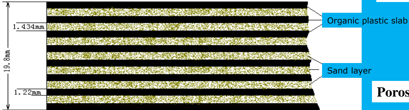
Scaled schematic map of thin interbedded model
